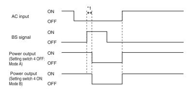
(2) When BS signal is used to shut down the UPS when AC input is ON
